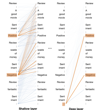
Figure 1: Visualization of the information flow in a GPT model performing ICL. The line depth reflects the significance of the information flow from the right word to the left. The flows involving label words are highlighted. Label words gather information from demonstrations in shallow layers, which is then extracted in deep layers for final prediction.
